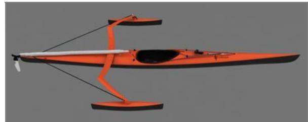
**Figure 8** New design of a sailing kayak: folded rig, paddling position.
