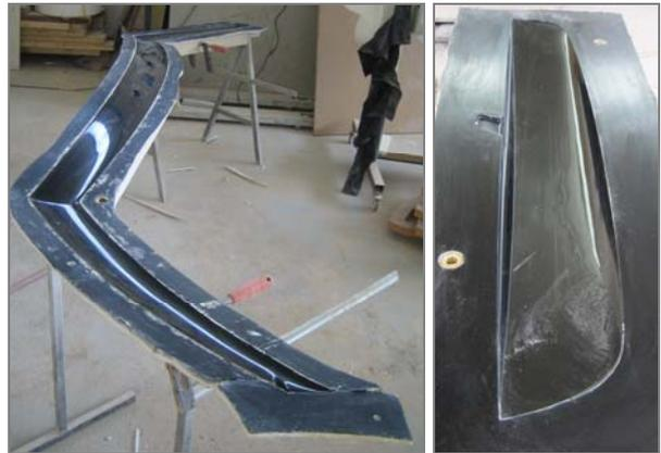
**Figure 14** Moulds for the crossbar and the outriggers.
