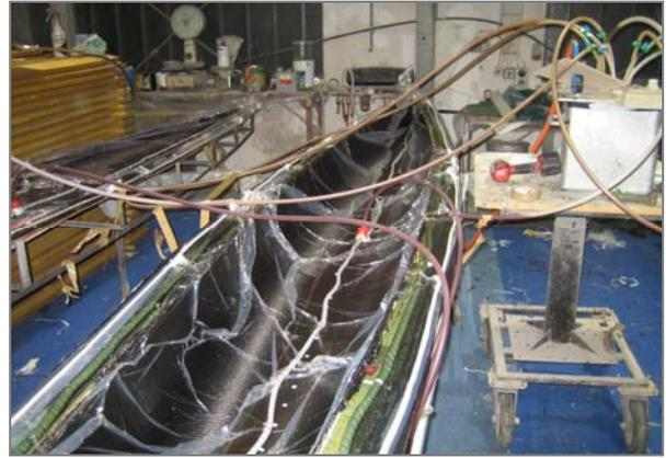
**Figure 13** Vacuum infusion of a main hull.
